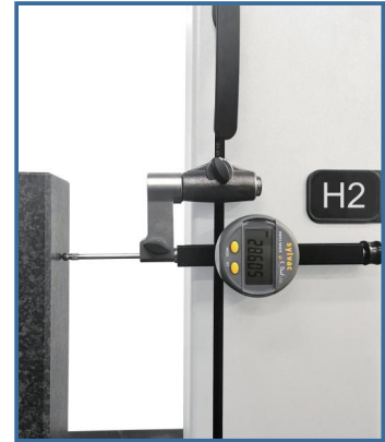
Electronic probe for measuring squareness
